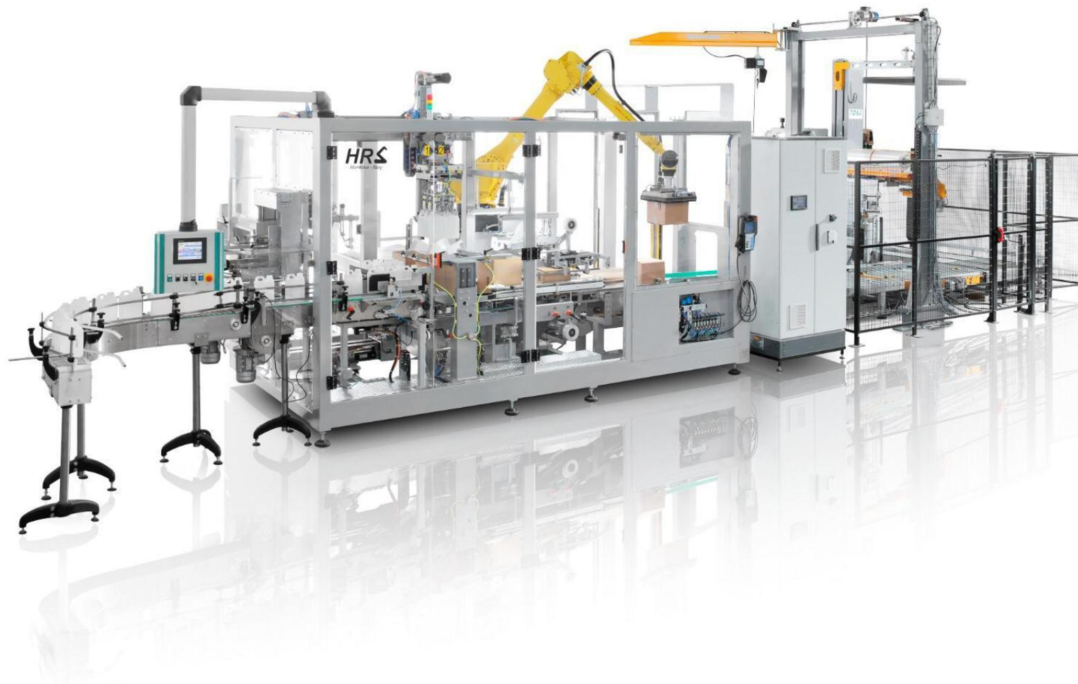
*Multifunction Robot Block MRB - with cartesian axes device and pallet stretch wrapping*
