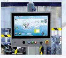
18" touch screen to control and regulate the labeller with built-in quality control.
