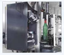
Vision Control: a quality control system enabling the precision of the pack to be verified and faulty containers to be re-
