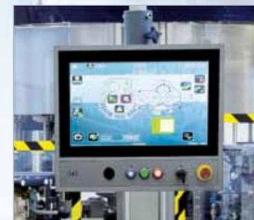
18" touch screen to control and regulate the labeller with built-in quality control.
