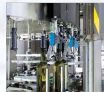
The **Follower** optical guide system (an exclusive Makro patent) enables the bottles to be aligned for application of labels in precise positions with respect to a reference on the bottle and reduces format change times. It is available in carbon fibre and fitted with a line scan camera.
