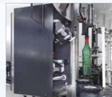
Vision Control: a quality control system enabling the precision of the pack to be verified and faulty containers to be rejected.
